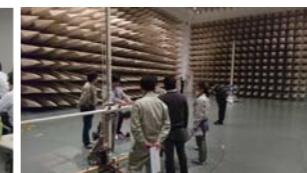
Hands-on training for antenna calibration
